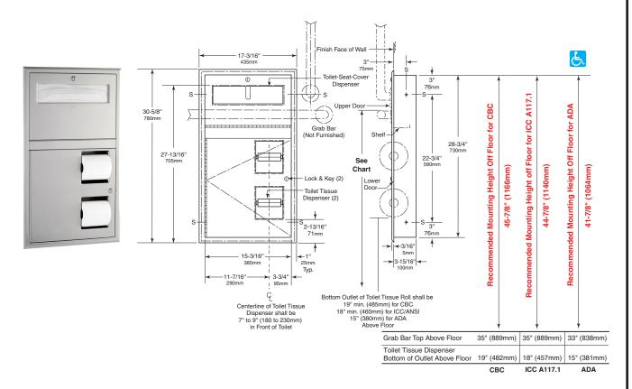
**Note:** For accessible toilet compartments, please use horizontal recessed or surface -mounted combination dispenser-/disposal-units, B-3091 or B-3092 Series, to comply with ADA 1-1/2" absolute Grab Bar wall spacing.
