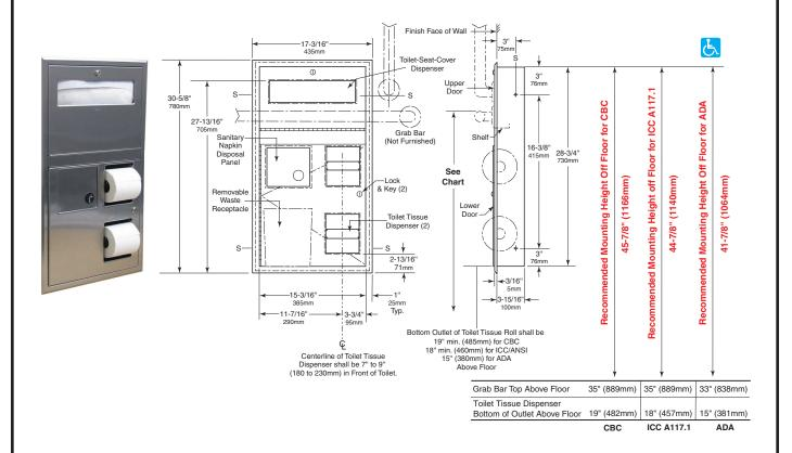
**Note:** For accessible toilet compartments, please use horizontal recessed or surface -mounted combination dispenser-/disposal-units, B-3091 or B-3092 Series, to comply with ADA 1-1/2" absolute Grab Bar wall spacing.
